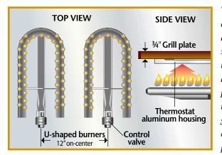
The U-shaped burner design covers more surface area than conventional straight burners. Heat is more evenly and widely distributed under the grill plate, allowing you to maximize the use of the grill surface for better consistency and productivity.
